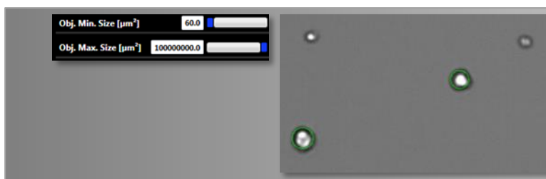
Fig. 23: Obj. Min Size 60 \mu\text{m}^2 The 2 vesicles are undetected because of their small size.
